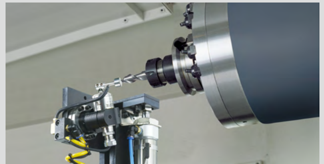
Automatic tool measuring device (TS 27R) option
