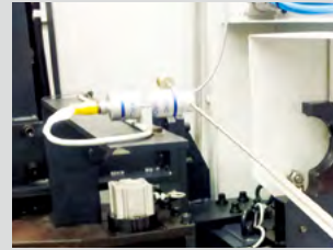
Auto tool damage detection device I (BK 9) option
