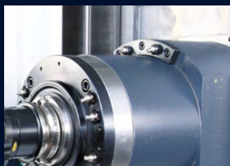
Coolant spray gun on the spindle head
